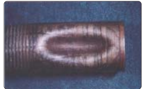
Fig. 6. Collapse of evaporator tube because of freeze-up.
