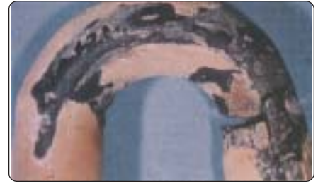
Fig. 4. Thermal Fatigue Failure in U-bend.
