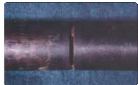
Fig. 3. Velocity-induced vibration of tube.
